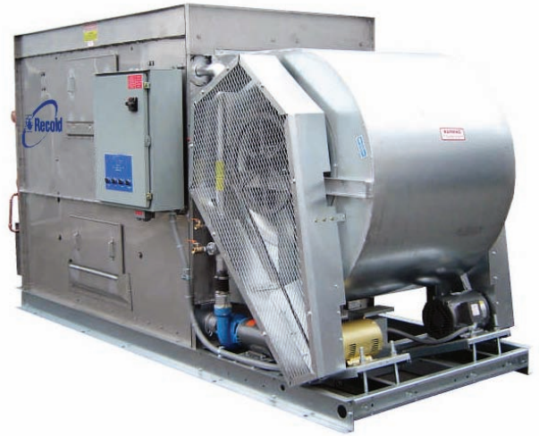
Recold JT Cooling Tower —Forced-draft, low profile design. G-600 galvanized steel factory assembled structure. Also available in 300 series stainless steel. Capacities from 135 to 1815 kW per cell.
